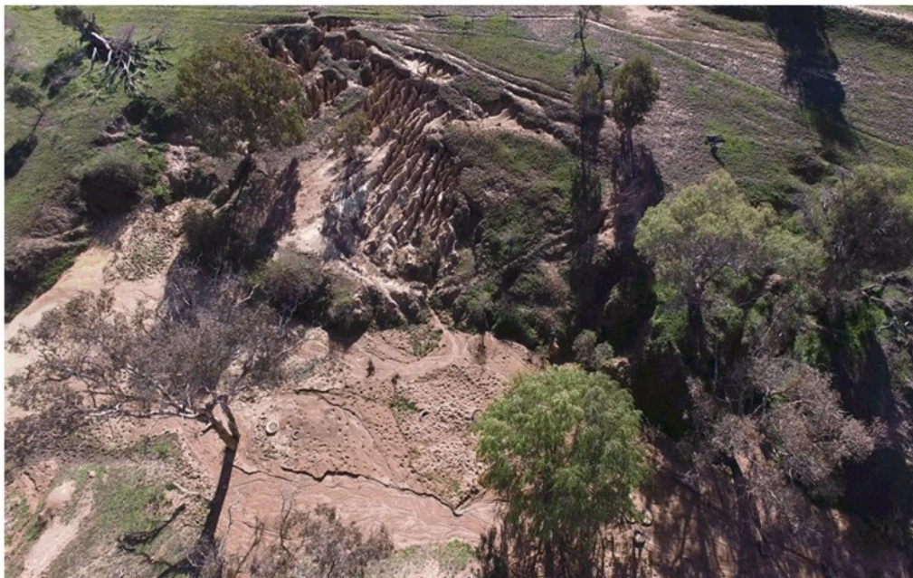
Photo 3: Severely eroding gully sidewalls - sediment deposited in channel from upslope erosion
