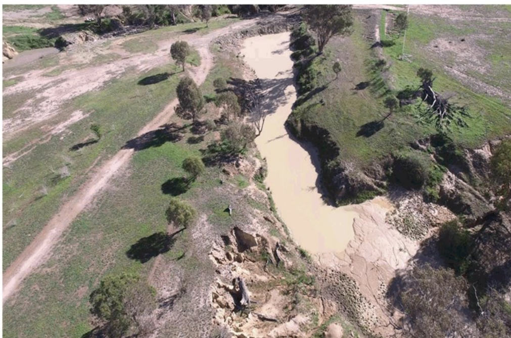
Photo 1: Downstream dam with high suspended sediment load
