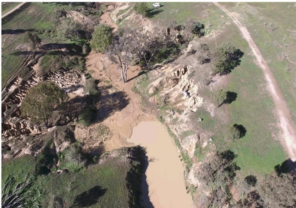
Photo 2: Deposited sediment in dam backwaters
